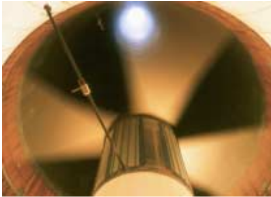
Fig. 5. The turbine of the prototype plant in Manzanares.
