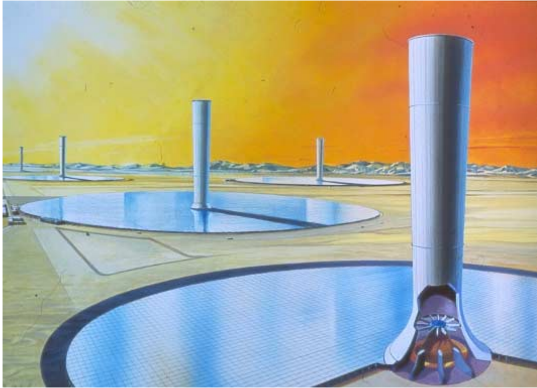
Fig. 10. Artist view of the essential components of a solar chimney: the collector, a flat glass roof (the chimney, a vertical tube supported on radial piers, and the wind turbines at the chimney base).
