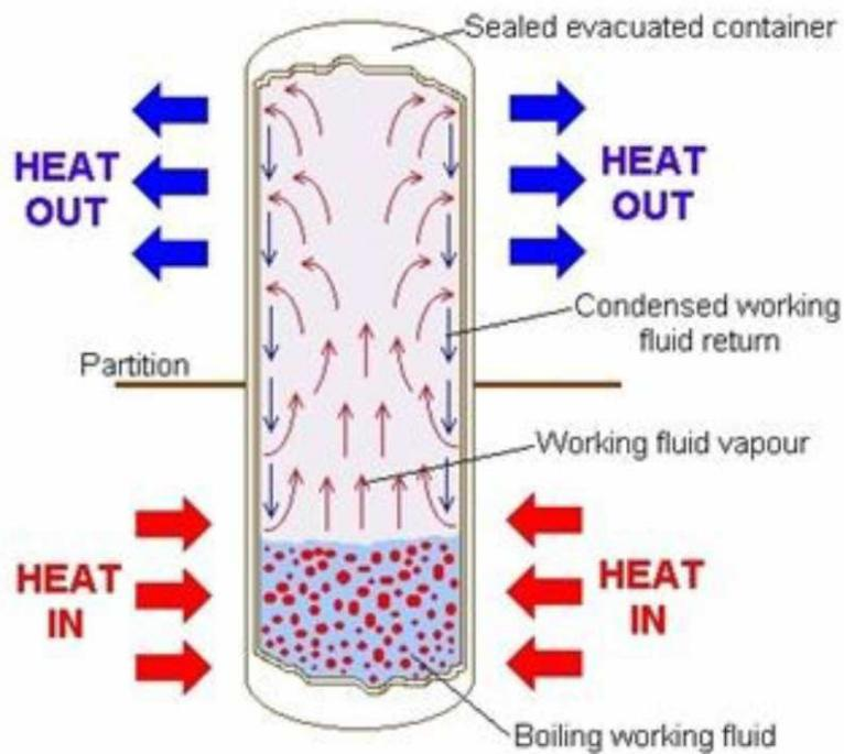
Schematic Representation of the Heat Pipe
